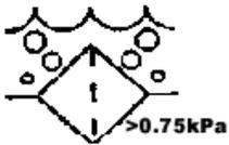
Fabrication integrity (or bubble point) is determined by the ISO 2942 test procedure. This test ensures that the filter media does not leak due to holes or improper assembly. In this test, the filter element is submerged in test fluid and slowly pressurized until bubbles appear.
