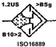
Capacity/efficiency can be determined from ISO 16889 Multi-pass test procedure. This test will tell you how much contaminant the filter will retain and the efficiency of the filter in removing the contaminant. This is a laboratory test that is very difficult to compare to the real world, but it will give a relative comparison of different filters, if the test conditions are the same. The capacity is usually given in grams of standardized test contaminant. The efficiency is given as a Beta ratio.
