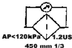
Resistance to flow or differential pressure shows how pressure drop occurs across the filter or how much resistance to flow the filter imparts to the system. This resistance, sometimes referred to as pressure drop or delta P ( $\Delta P$ ), has a direct bearing on the filter life. Be sure you note the viscosity and flow of the fluid used in determining these criteria.
