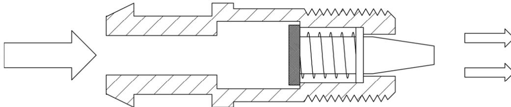
At high speeds manifold vacuum is decreased. The plunger is only drawn to a point about midway in the housing. This allows a maximum flow of vapor. Since the engine needs more fuel/air mixture at high speeds, the introduction of more vapor does not affect performance. In the event of a backfire, pressure from the intake manifold forces the plunger to the closed or engine-off position. This prevents the backfire flame from reaching the crankcase and exploding the combustible vapor.
